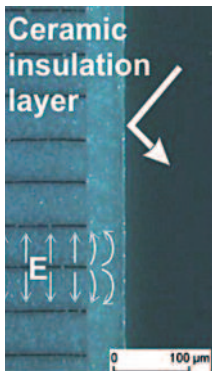
Fig. 1: The ceramic insulating layer prevents the ingress of water molecules and reliably protects the sensitive internal electrodes from mechanical damage and dirt
